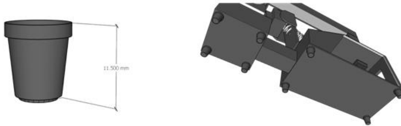
Figure 9. Footing placement. The footing has rubber in it to maintain the stability of the device while testing watermelons.
