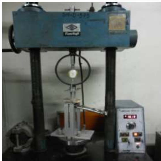
Figure 5. Face Screw Holding Test Set – Up
