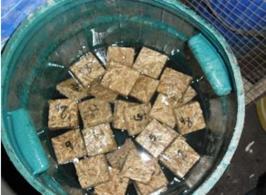
Figure 3. Soaking of Specimen in Water
