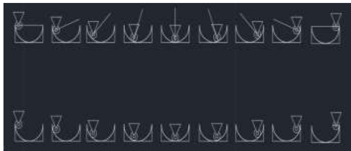
Figure 8. Self-righting diagram of the base isolation installed in one of the structural models.
