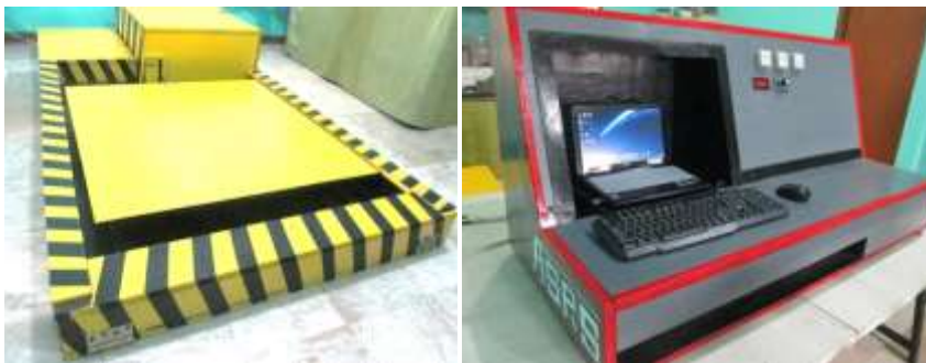
Figure 2. A fully operational Titan earthquake shake table (left) and its control board (right).
