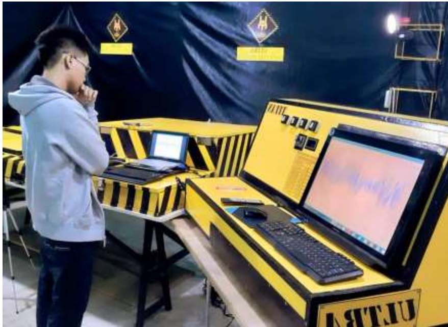
Figure 3. Ultra Construction Innovators' head researcher runs a calibration test on the newly improved control board of the the third prototype of the Titan earthquake shake table.
