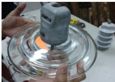
Figure 2. Model of LXWP4-70 glass suspension insulator.
